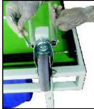
Attach long brace support P2 & small brace support P3 with wheel assembly P4 using nut and bolt P22 - 100x8mm and tighten it with the help of two spanners.
