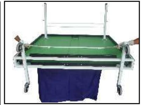
Attach wheel assembly P4 with cross pipe P5 using nut and bolt P23 - 90x8mm at both ends and tighten it with the help of two spanners.
