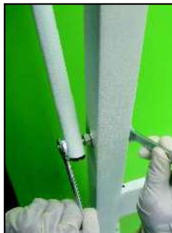
Attach long brace support P2 with outer leg P1 using nut 8mm and tighten it with the help of two spanners.
